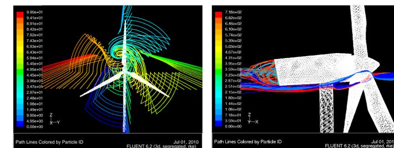
Fig. 3: Pathlines of particles and turbulence around the nacelle.
