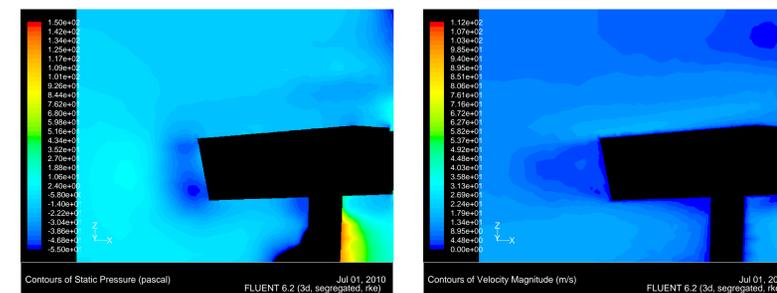
Fig. 2: Pressure and velocity on the nacelle.
