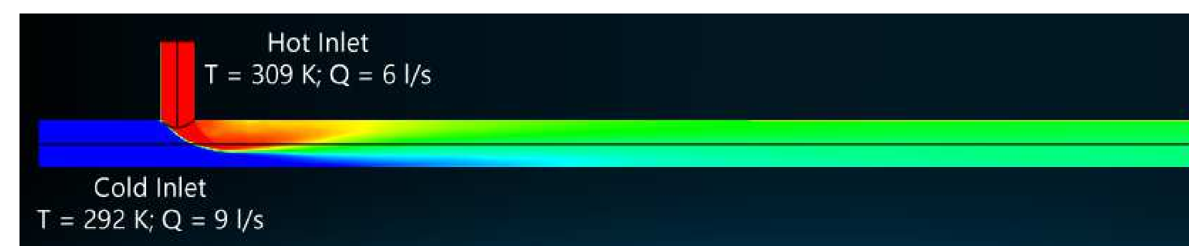
Fig. 1: Overview of the T-Junction simulation. Averaged temperature field after 16s.
