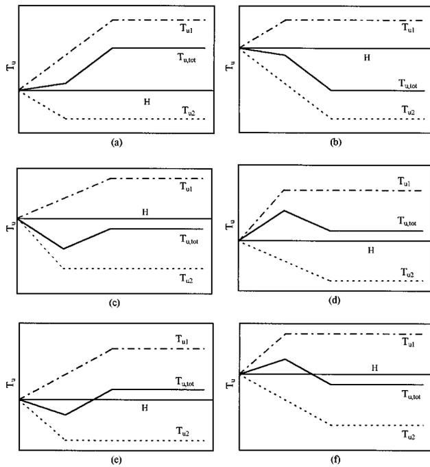
FIG. 3. Linear approximation of the evolution of the amplitude of the torque curves with the applied magnetic field in samples with two zones I and II affected by mutually perpendicular uniaxial magnetic anisotropies for different cases.  $T_{u1}$ ,  $T_{u2}$ , and  $T_{u,tot}$  indicate the amplitude of the uniaxial component of the torque curves corresponding to zones I, II, and the whole sample, respectively.
