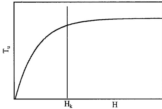
FIG. 1. General evolution of the amplitude of the torque curves,  $T_u$ , with the applied magnetic field,  $H$ , in amorphous magnetic materials.
