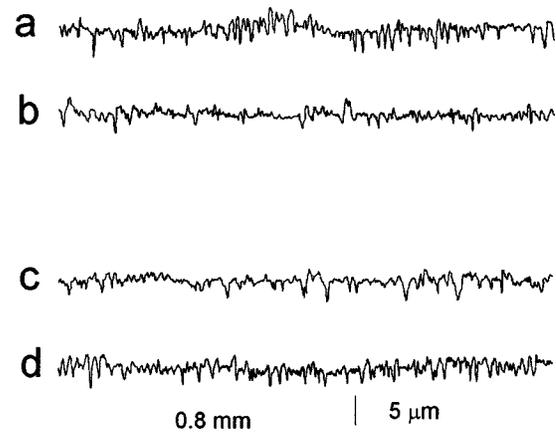
FIG. 4. Surface profiles of the wheel surface of samples of Vitrovac 6150: (a) and (b) profiles along the transversal and longitudinal direction in the majority of the ribbon, (c) and (d) the same as (a) and (b) but in the parts affected by the anomalous behavior of the torque measured.
