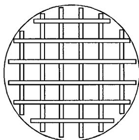
FIG. 5. Distribution between the strips (0.45 mm width and 23  $\mu\text{m}$  thick) of  $\text{Co}_{73.5}\text{Ni}_3\text{Cu}_1\text{Si}_{13.5}\text{B}_9$  in the sample simulating the surface roughness. Diameter of the sample 13 mm, spacing of the strips 1.5 mm.
