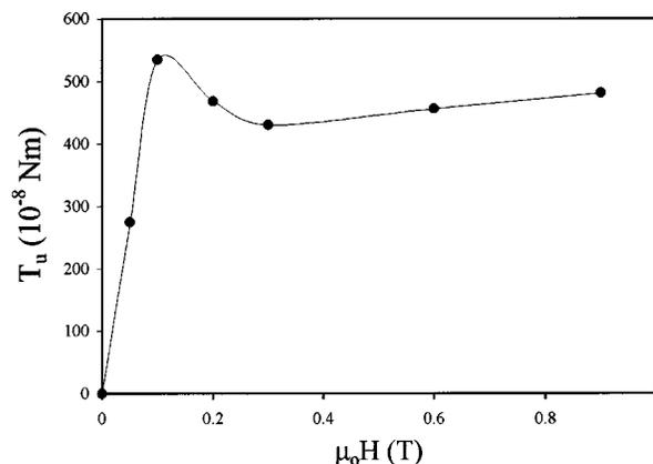
FIG. 6. Experimental evolution of the amplitude of the torque curves  $T_u$  of the sample of Fig. 5 with the applied magnetic field  $\mu_0 H$ .
