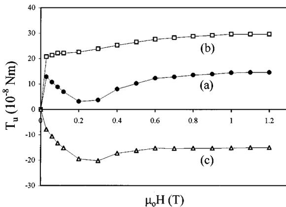
FIG. 2. Experimental evolution of the amplitude of the torque curves  $T_u$  of Vitrovac 6150 with the applied magnetic field  $\mu_0 H$ , in: (a) as-quenched samples, (b) after mechanical polishing, and (c) curve resulting from the subtraction of curves a and b.
