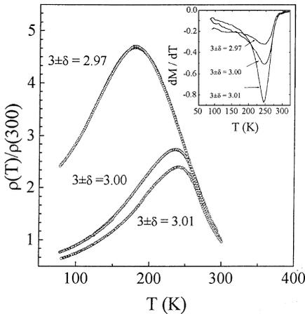
Fig. 1. Temperature dependence of normalized resistivity for reference and reduced samples. Oxygen stoichiometry is indicated.  $T_c$  does not follow  $T_{M-1}$  displacement with oxygen content (inset).
