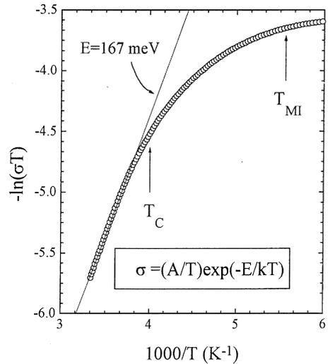
Fig. 2. Conductivity of  $3 \pm \delta = 2.97$  sample in the adiabatic limit. The adjustment of high temperature data gives an activation energy of 167 meV for the hopping motion. Note also the separation near  $T_c$ , which indicates higher electron mobility in the insulating range between  $T_c$  and  $T_{MI}$ .
