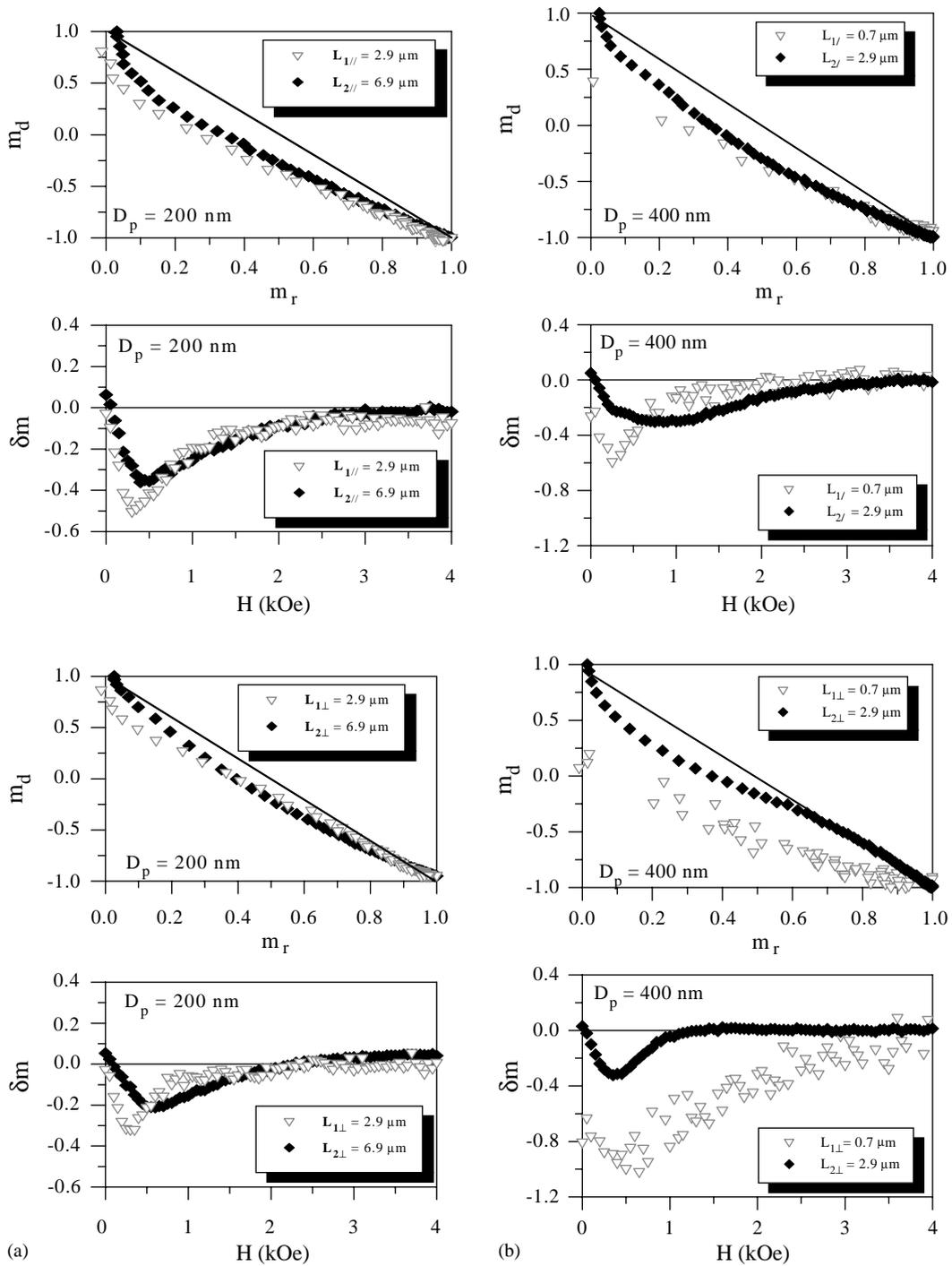
Fig. 3. Normalized remanent curves and  $\delta m$  plots for Co wires of (a) 200 and (b) 400 nm in diameter with the applied field perpendicular and parallel to the wire axis for short ( $\nabla$ ) and long wires ( $\blacklozenge$ ).
