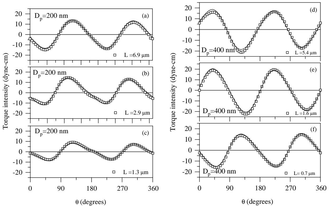
Fig. 4. Measured ( $\square$ ) and calculated (—) torque intensity curves at room temperature of a series of arrays of Co wires with (a–c) 200 and (d–f) 400 nm diameters as functions of wire lengths, with (a)  $L = 6.9 \mu\text{m}$ , (b)  $L = 2.9 \mu\text{m}$ , (c)  $L = 1.3 \mu\text{m}$  and, (d)  $L = 5.4 \mu\text{m}$ , (e)  $L = 1.6 \mu\text{m}$  and (f)  $L = 0.7 \mu\text{m}$ , respectively.
