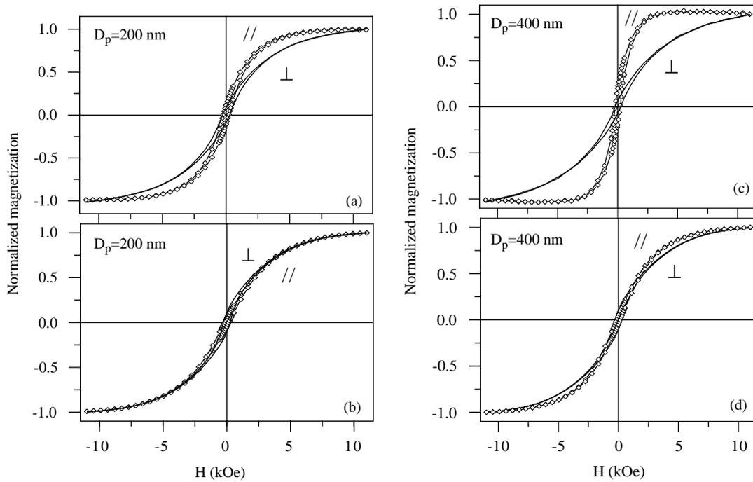
Fig. 1. Normalized hysteresis loops at room temperature of arrays of Co nanowires of (a, b) 200 and (c, d) 400 nm—diameters as a function of wire lengths, recorded with the field applied parallel (—◇—) and perpendicular (—) to the wire axis for (a, c) short wires and (b, d) long wires.
