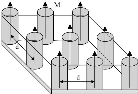
Fig. 2. Square dipolar arrays of Co wires with a lattice spacing  $d$ , when the magnetization is parallel to the wire axis.
