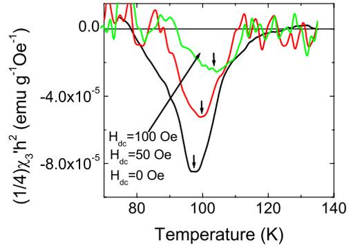
Fig. 6. The real part of the cubic term of the susceptibility vs. temperature for a field cooled sample (the superimposed DC field is indicated).
