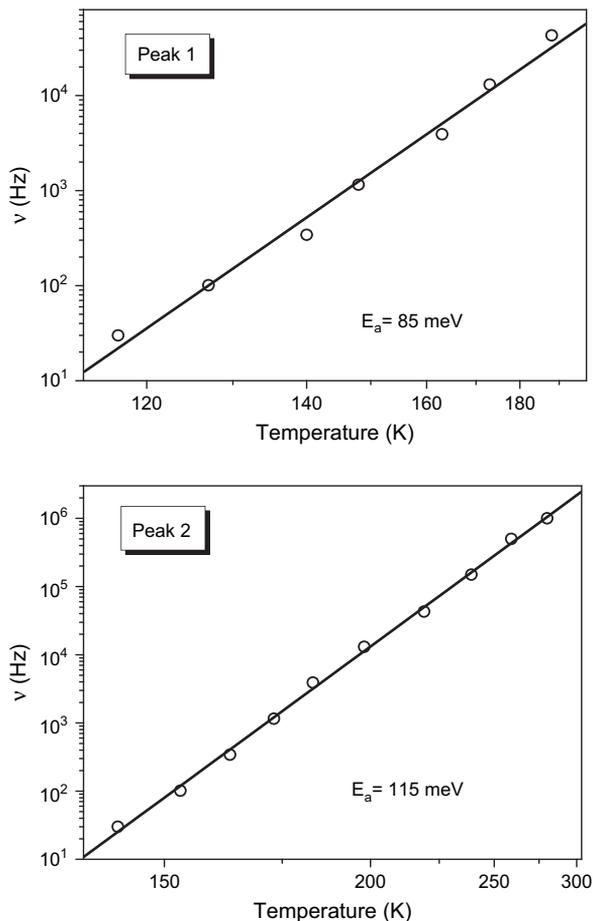
Fig. 3. Example of the Arrhenius plot of the shift of the two peaks as a function of frequency (sample of thickness 0.65 mm).
