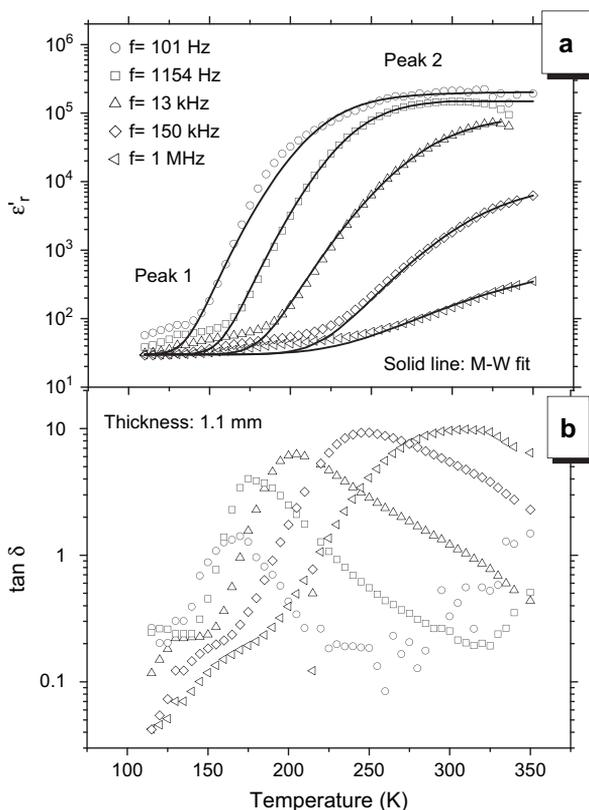
Fig. 1. (a)  $\epsilon'_r$  vs  $T$  curve obtained at several frequencies for the sample of thickness 1.1 mm. The solid lines represent the fit to the M–W model. (b) Corresponding  $\tan \delta$  vs  $T$  curve.
