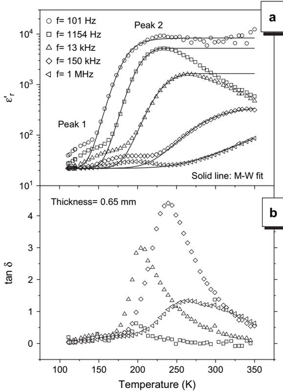
Fig. 2. (a)  $\epsilon'_r$  vs  $T$  curve obtained at several frequencies for the sample of thickness 0.65 mm. The solid lines represent the fit to the M–W model. (b) Corresponding  $\tan \delta$  vs  $T$  curve.
