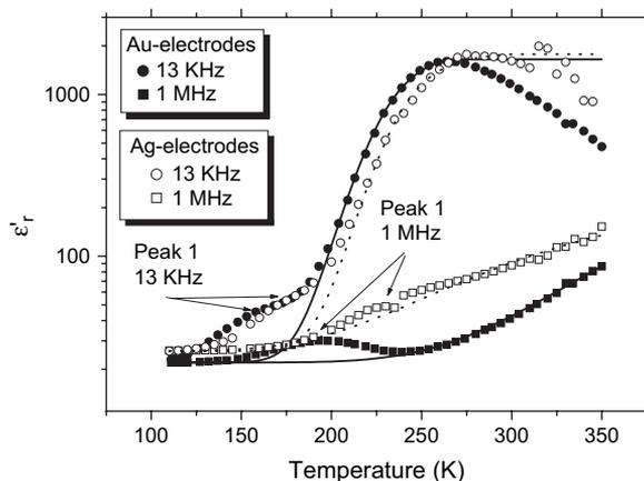
Fig. 6. Examples of  $\epsilon'_r$  vs  $T$  curves obtained at 13 KHz and 1 MHz using two different electrode contacts: sputtered gold and sputtered silver (sample of thickness 0.65 mm).
