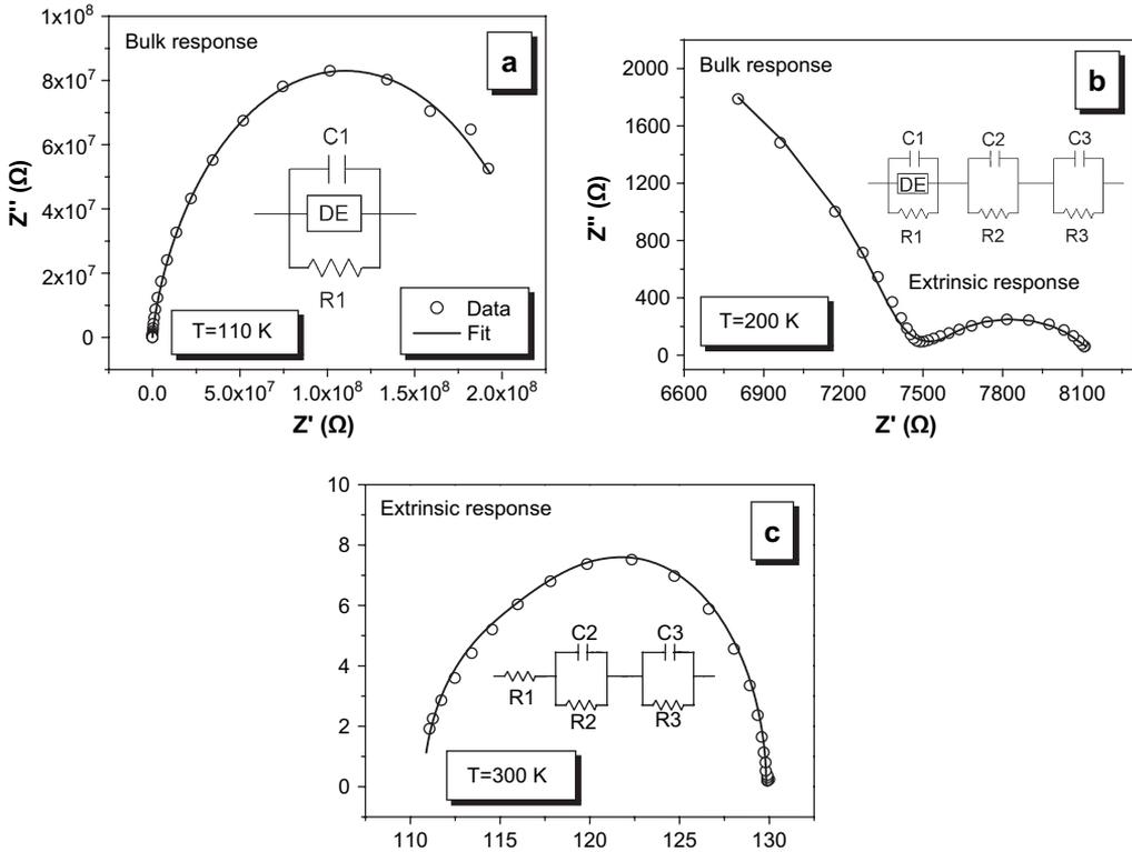
Fig. 4. Impedance complex plane plots and equivalent circuits obtained for the  $\text{CaMn}_7\text{O}_{12}$  compound (sample of thickness 1.1 mm) at three different representative temperatures (110, 200 and 300 K).
