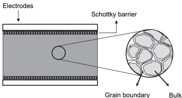
Fig. 5. Schematic representation of the three different regions proposed to explain the dielectric behavior obtained for this compound.
