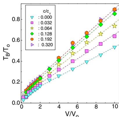
**Fig. 1.** Reduced blocking temperature,  $T_B/T_0$ , as a function of the particle size,  $V/V_0$ , for different particle concentrations,  $c/c_0$ .
