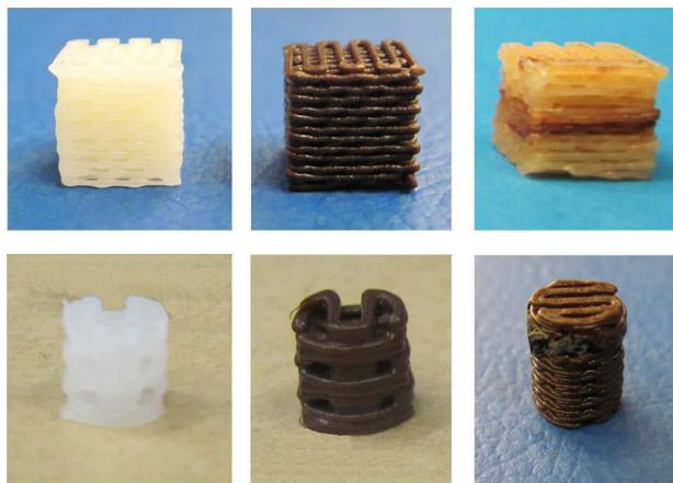
Fig. 5. PCL and nanocomposite scaffolds for bone tissue engineering. Top line: cubic scaffolds made of PCL, PCL/FeHA 80/20, and gradient PCL/FeHA. Bottom line: cylindrical scaffolds made of PCL, PCL/FeHA 80/20, and gradient PCL/FeHA.
