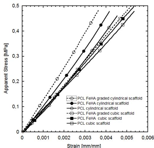
Fig. 6. Stress–strain curves at low-strain levels of cubic scaffolds made of PCL, PCL/FeHA 80/20, graded PCL/FeHA and of cylindrical scaffolds made of PCL, PCL/FeHA 80/20, graded PCL/FeHA.
