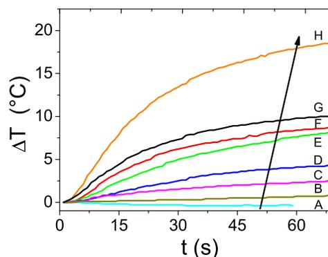
Fig. 3. MH curves for gelatin-based scaffolds containing increasing MNPs loadings from A to H, as indicated by the arrow.
