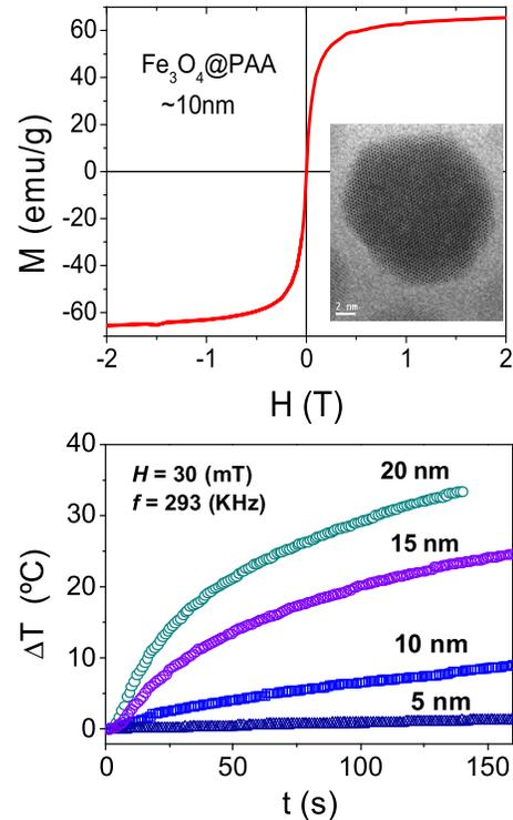
Fig. 1. Top: SPM curve of  $Fe_3O_4@PAA$  MNPs. Inset shows a TEM image of one single particle. Bottom: particle size dependence of MH of  $Fe_3O_4@PAA$  MNPs.
