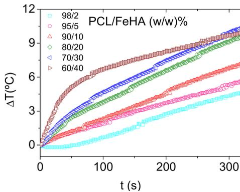
Fig. 7. Hyperthermia curves of magnetic PCL-based scaffolds at several PCL/FeHA concentrations and with cubic structure. The frequency and magnetic field of the generated oscillating magnetic field were 293 kHz and 30 mT, respectively.
