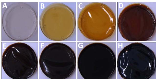
Fig. 2. Gelatin-based magnetic scaffolds with increasing loading of  $\text{Fe}_3\text{O}_4$ @PAA MNPs from A to H.
