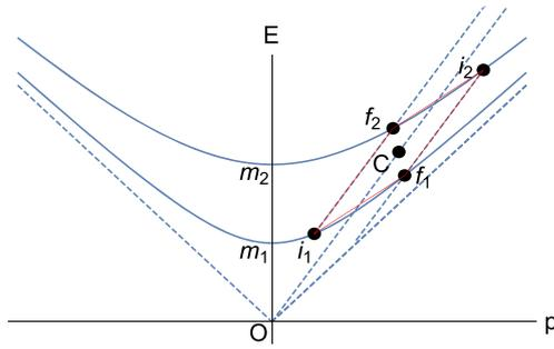
**Figure 2.** Kinematic solution of a relativistic one-dimensional elastic collision in an arbitrary inertial frame. The initial momentum and energy of the colliding bodies are represented by  $i_1, i_2$  and the final ones by  $f_1, f_2$ . The point C is the centre of the parallelogram connecting them.
