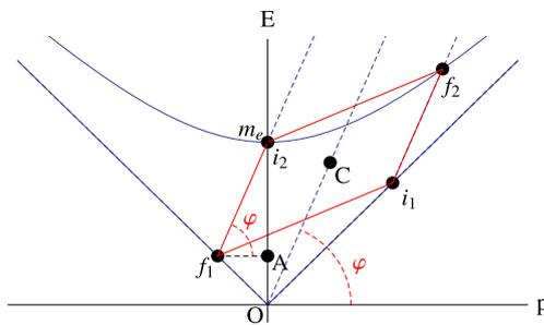
**Figure 3.** Kinematic solution of an example of one-dimensional Compton scattering. The auxiliary point A is placed at  $p_A = 0, E_A = |p_{f1}|$ .
