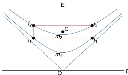
**Figure 1.** Kinematic solution of a relativistic one-dimensional elastic collision in the centre of mass frame. The initial momentum and energy of the colliding bodies are represented by  $i_1$ ,  $i_2$  and the final ones by  $f_1$ ,  $f_2$ . The point C is the centre of the rectangle connecting them. The two hyperbolas, parameterised by the masses  $m_1$  and  $m_2$  correspond to the dispersion relation of (1).
