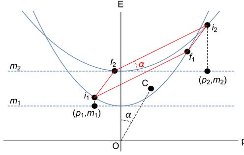
**Figure 4.** Kinematic solution of a non-relativistic one-dimensional elastic collision. The initial momentum and energy of the colliding bodies are represented by  $i_1, i_2$  and the final ones by  $f_1, f_2$ . The point C corresponds to  $(\frac{1}{2}(p_1 + p_2), \frac{1}{2}(m_1 + m_2))$ . The two parabolas, parameterised by the masses  $m_1$  and  $m_2$  correspond to the dispersion relation of (1), where  $\text{const} = m$  has been chosen.
