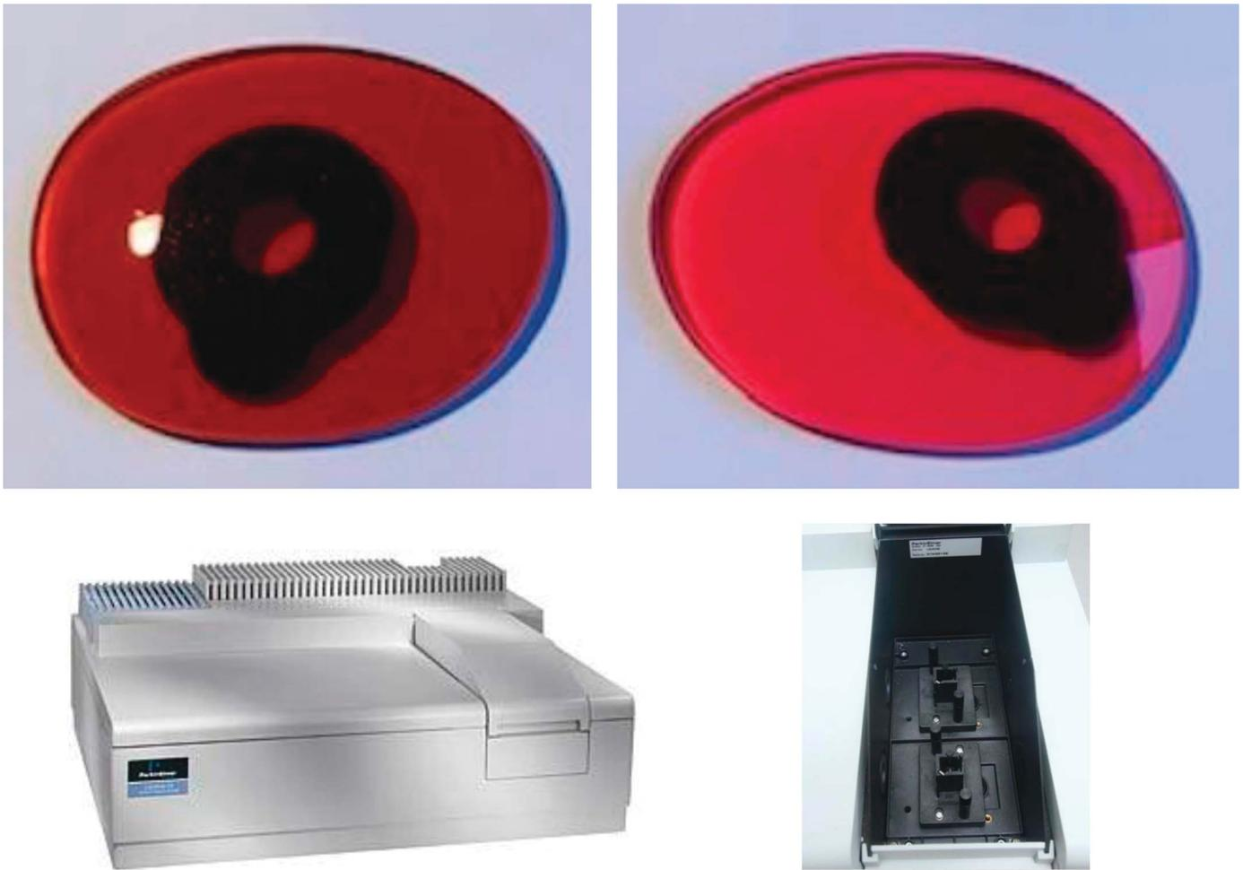
**FIGURE 2.** ChromaGen haploscopic filters (top) marked to be analyzed with the PerkinElmer Lambda 25 UV/Vis spectrophotometer (bottom).
