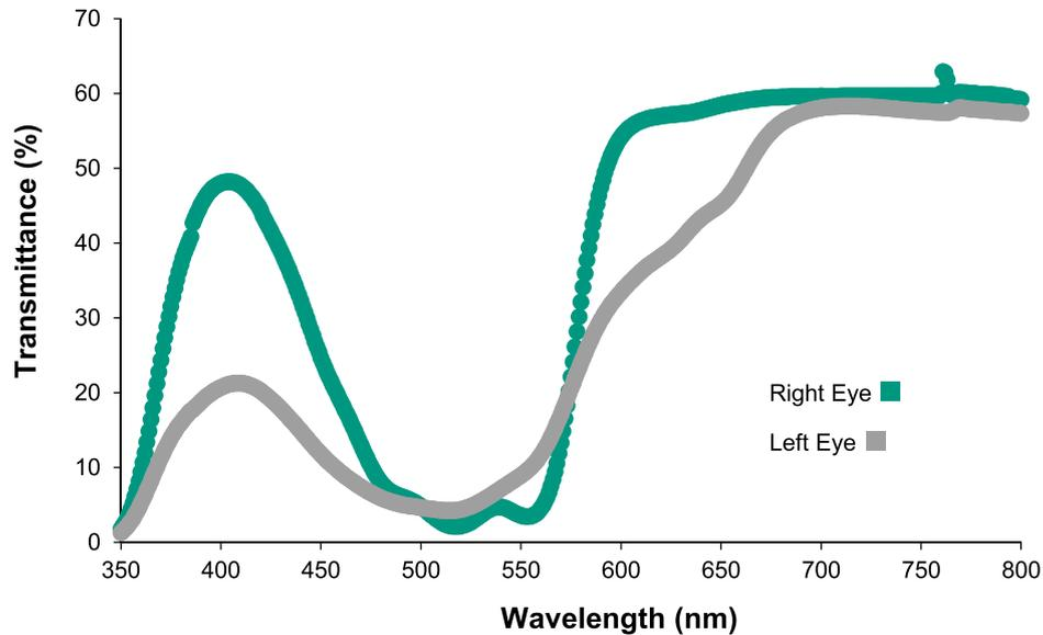
**FIGURE 3.** ChromaGen lens transmittance analysis of the right and left filters used in this study. Note the asymmetric configuration around the confusion axis.
